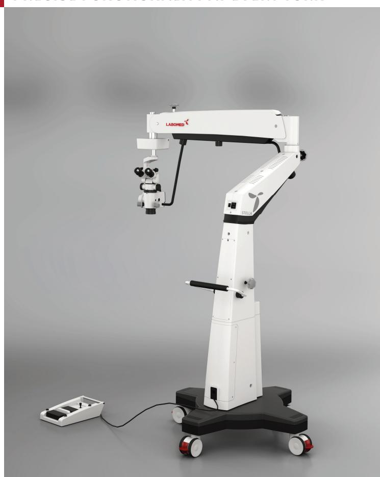
Stella provides surgeons a waterproof foot control (10-way) that will effortlessly drive X, Y, and Z axis motors alongside mag change and light intensity adjustment functions. Conveniently housed in the arm system is an IR and UV safe LED (6500 kelvin) that will provide cool, crisp and bright-white illumination (rated 60,000 hours of LED life).
