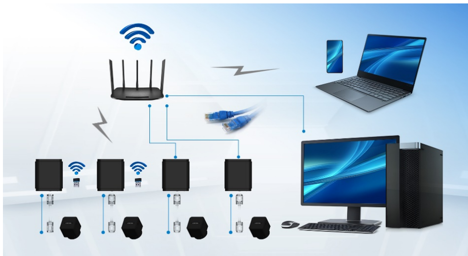
Fig. 7 — Mixed wired and wireless deployment. Two cameras are connected by Ethernet; two are connected by Wi-Fi STA. All hosts read from the same router.
