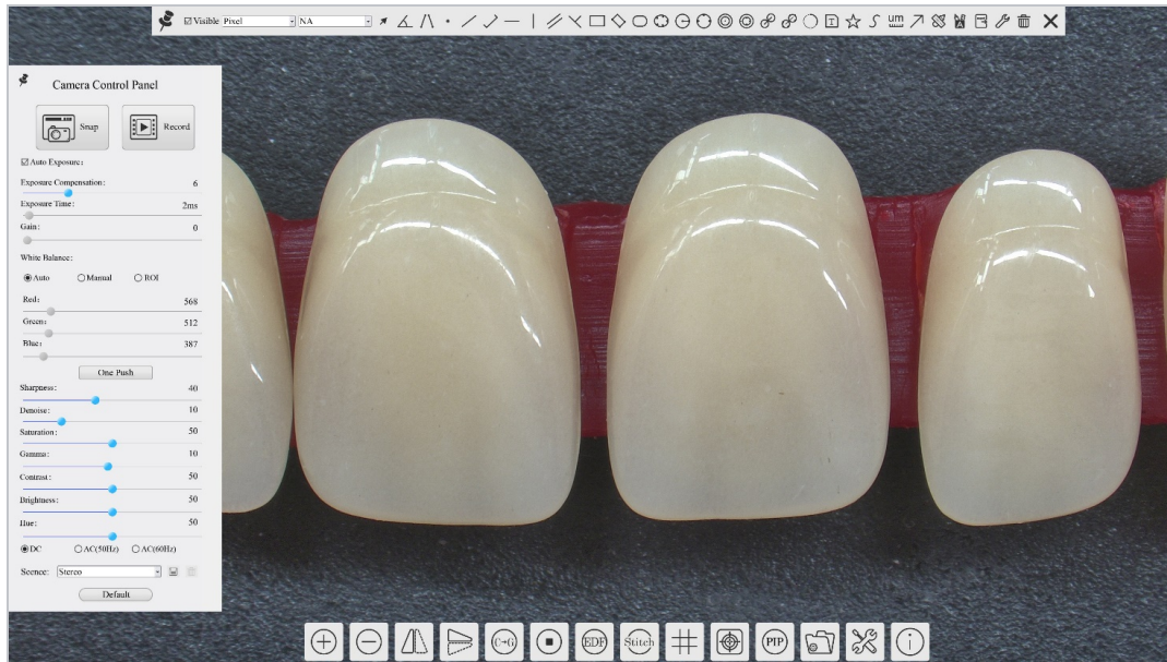
Fig. 8 — The embedded Atlas+ 4K interface. Camera Control Panel at left; Measurement Toolbar at top; Synthesis Camera Control Toolbar at bottom.
