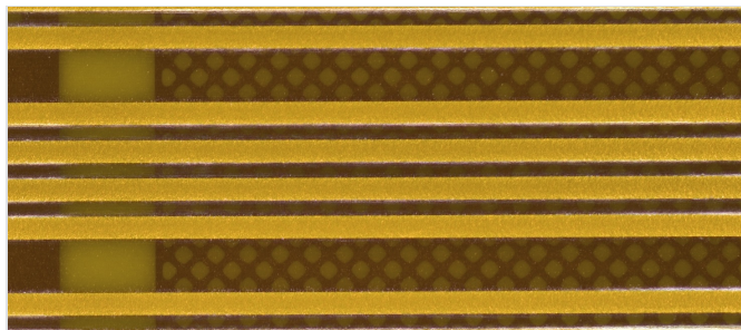
Fig. 11 — Conductive traces on a flexible printed circuit.
