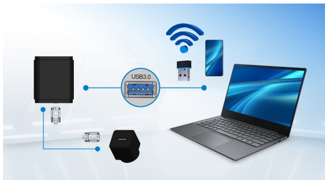
Fig. 5 — In Wi-Fi AP mode, the master device hosts the wireless network. Hosts join the network directly.
