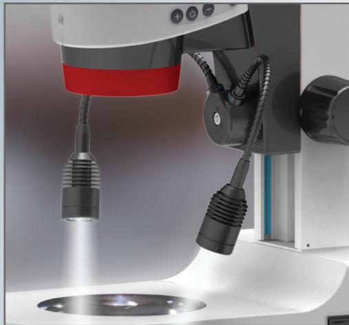
The Luxeo 6Z allows users to choose an ultra-bright front mounted gooseneck arrangement that efficiently hides all wiring in the arm bracket, while keeping the goosenecks away from focus controls. This provides the user with hassle free control of indirect illumination angles. Ring light only options are also available.
